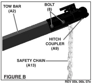
through the center link in the Safety Chain, and through the Tow Bar. Firmly tighten a Lock Nut (8) onto the Bolt (8) to secure the Safety Chain to the Tow Bar. Insert another Bolt (8) through the *side/rear* mounting holes of the Hitch Coupler and Tow Bar and secure with a Lock Nut (8). (See Figures A and B.)
